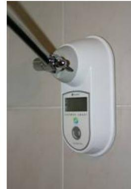
The block diagram of Figure 3 shows the key functional elements of the Smart Shower Meter. Careful software and electronics design achieved a service lifetime in excess of six months from two alkaline AAA cells.
