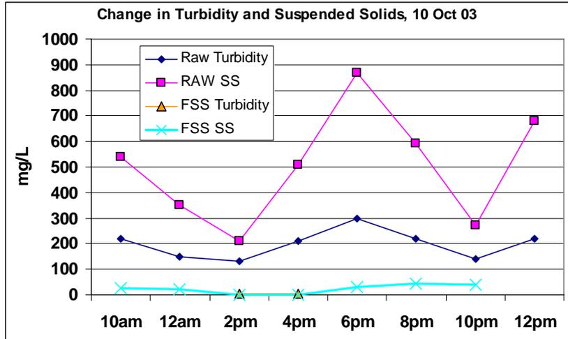
Fig. 7. Raw Sewage and FSS Effluent Turbidity and Suspended Solids, Brushy Creek, 10<sup>th</sup> October 2003
