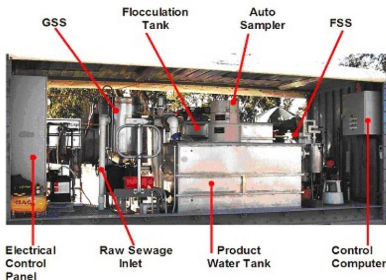
This report covers trials involving application of the FSS process to sewer mining by combining it with other downstream processes to produce a high quality effluent from raw sewage for reuse purposes.
