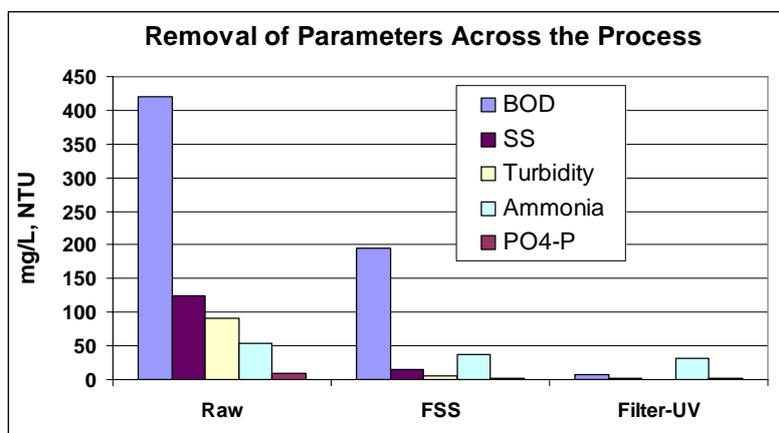
Fig. 10 Effect of treatment on the measured parameters.
