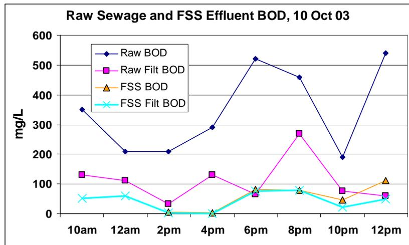
Fig. 5. Raw Sewage and FSS Effluent BOD
