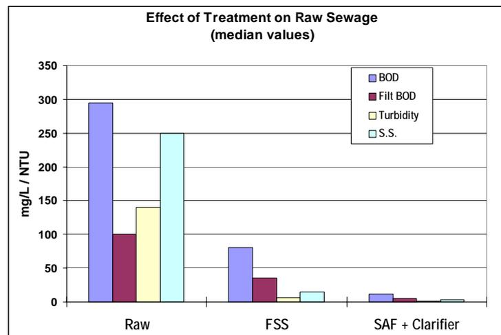
Fig. 4 Reduction in various water quality parameters across the process
