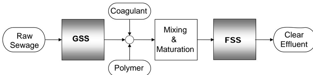
Fig. 2 Flowchart for the CDS Fine Solids Separation Process
