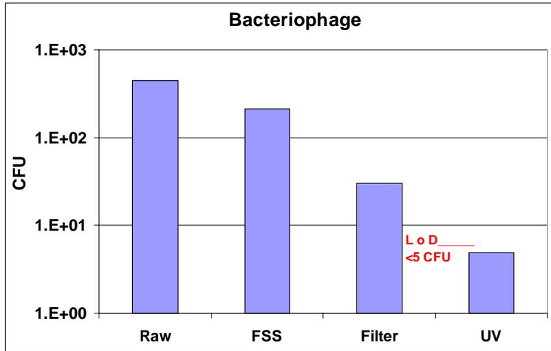
Fig. 11. Log reduction of bacteriophage across the process (LoD = limit of detection).
