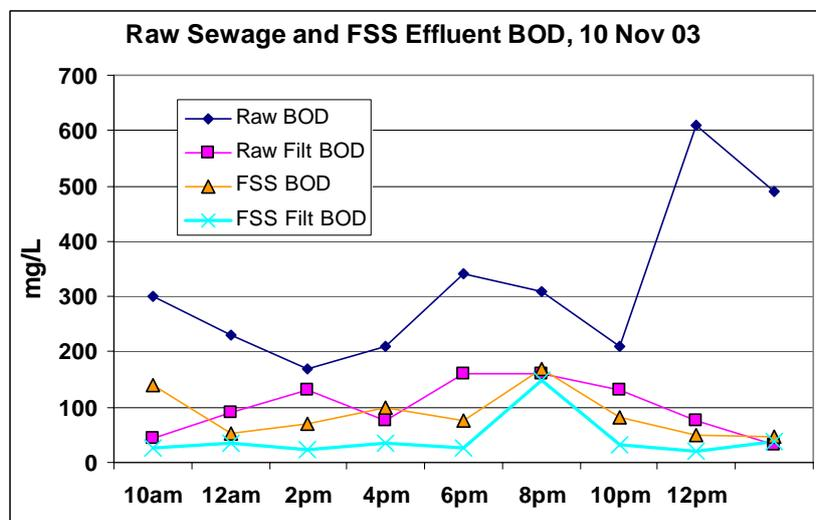
Fig. 6. Raw Sewage and FSS Effluent BOD
