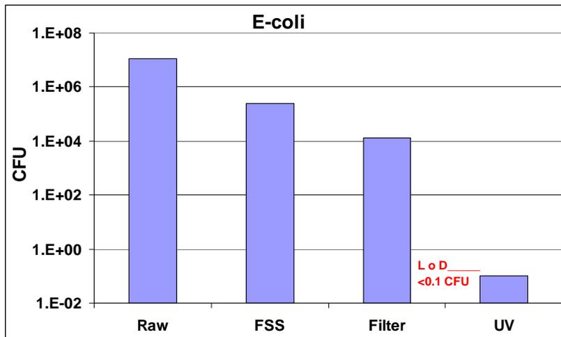
Fig. 12. Log reduction of E-coli across the process (LoD = limit of detection).
