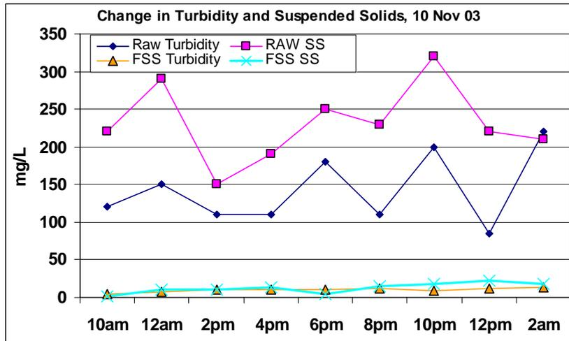
Fig. 8. Raw Sewage and FSS Effluent Turbidity and Suspended Solids, Brushy Creek, 10<sup>th</sup> November 2003
