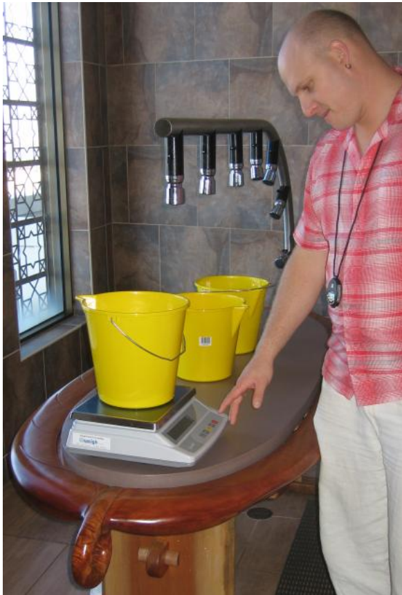
Figure 2 Measurement of water use by Vichy treatments (above) and other water uses
