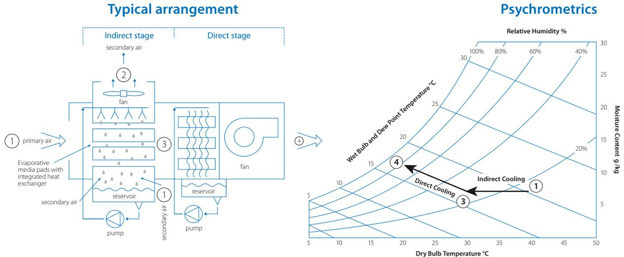
Secondary air enters indirect section at condition 1, and leaves wet pads at condition 2.
